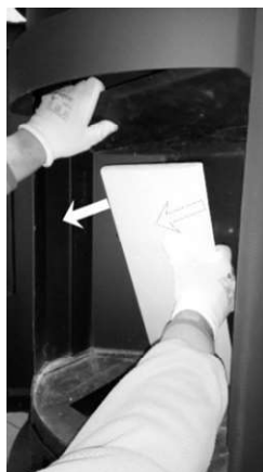
8. Pull out the rear concrete plate.
