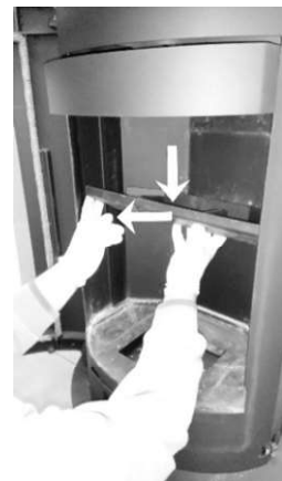
6. Push the metal deflector upwards, slightly turn the plate towards the centre of the fireplace.
