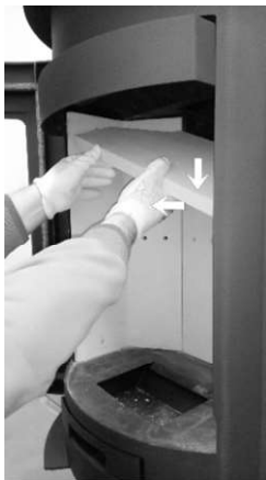
4. Slightly turn and slide out the concrete deflector.
