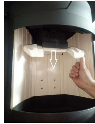
3. Drop and remove concrete deflector.
